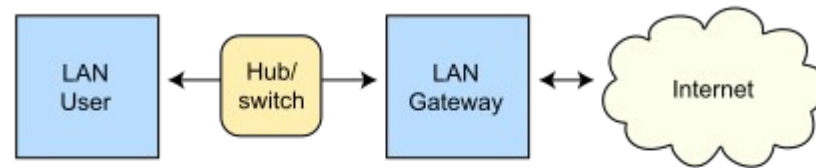
Routing under normal operation
